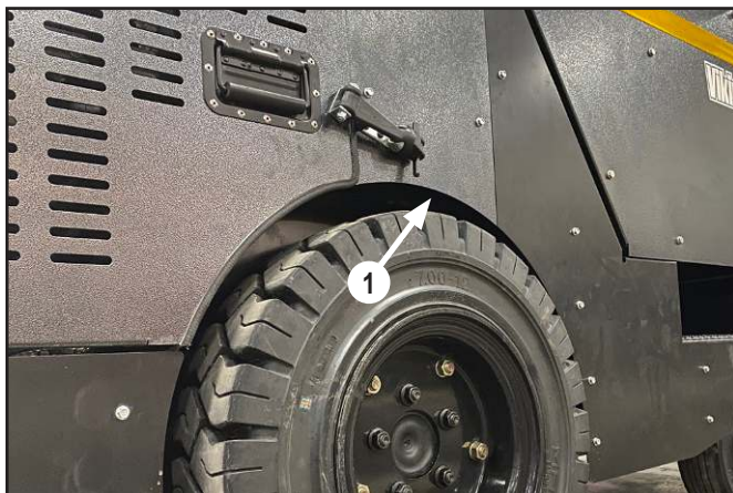
(1) Hydraulic oil drain plug
