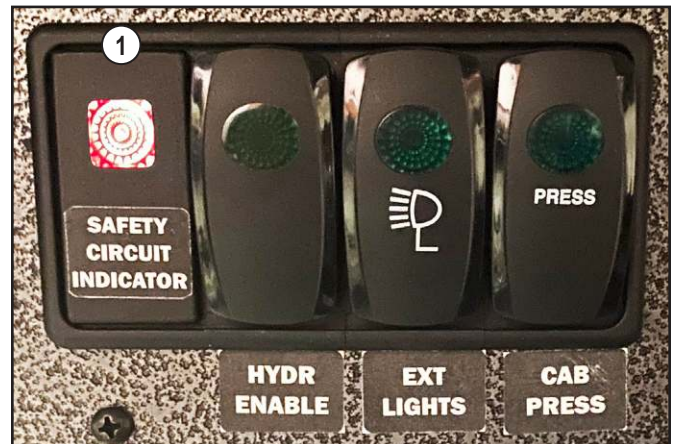
(1) Safety circuit indicator lit up indicating the hydraulic system is disabled.
