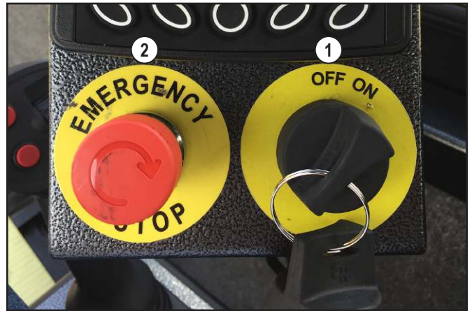
(1) Ignition switch (2) Emergency stop switch
