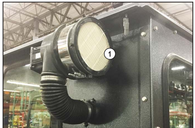
(1) Cab pressurizer air filter
