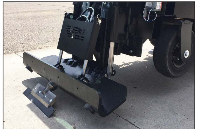
Increased (steep) blade tilt angle and lowered blade. Front caster wheels high off ground.
