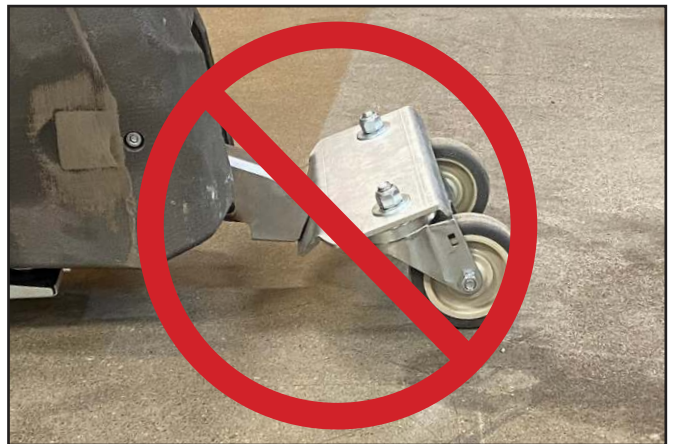
Poor maneuverability—bracket NOT parallel to floor.
