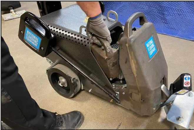
Removing middle weight.
