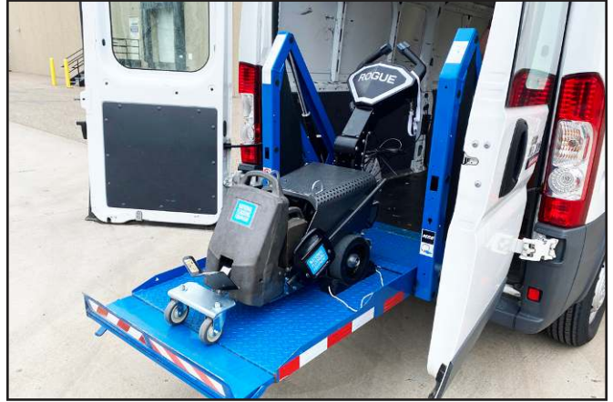
Transporting with power liftgate
