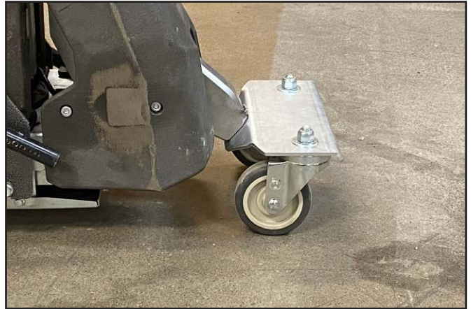
Good maneuverability—bracket parallel to floor.
