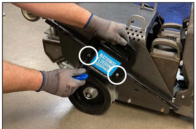
Adjusting slide weight.
