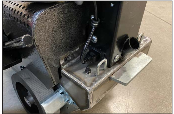
Proper slack in power cord
