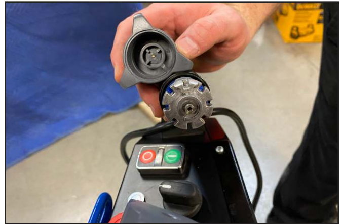
Control handle knob removed.
