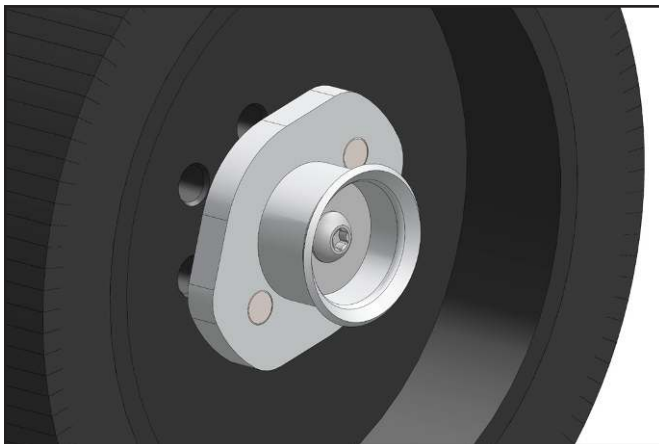
Wheel disengaged. Coupling flange is pulled out.
