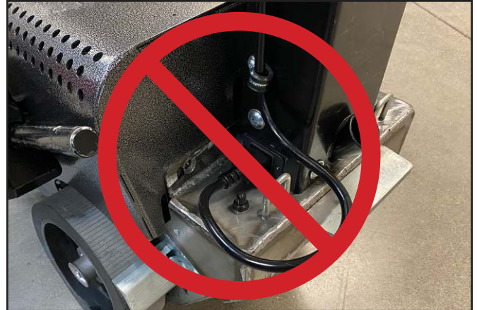
Power cord should NOT have excess slack.
