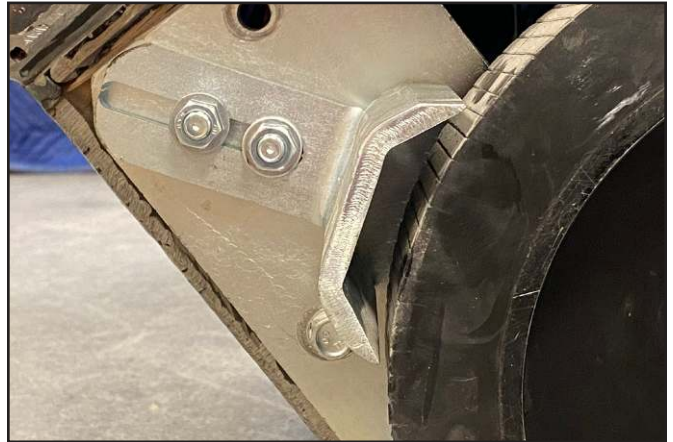
Wheel cleaner adjusted to proper gap.
