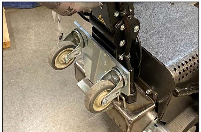
Proper orientation for transport wheels in stowed position
